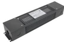
ELV-60J-24 1-60W driver ELV-80J-24 1-80W driver Class 2 dimming hardwire driver w/junction box, 60% minimum load; Dimming consumes ±3W internally
